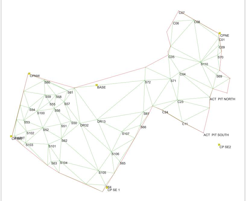
Topcon 3D Office created surfaces based on these point to point lines, their measurements, and elevations of the respective points. The 2 surfaces representing the top and bottom of pay, were compared by the software and a digital model of the pay formation was rendered. This model was calculated for volume and the results reported.
